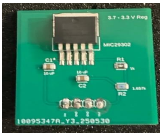
Figure.12. MIS29302-3.3 Voltage Regulator Board
